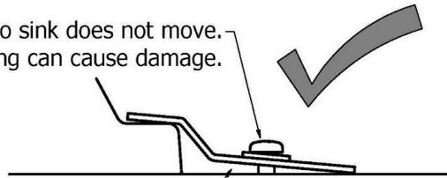
Hand tighten screw snugly so sink does not move.
